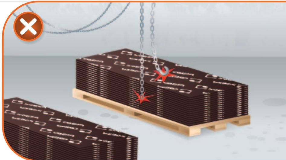
Remove sheets of plywood from the packs manually. Avoid damaging the flat ends, dropping plywood or dragging it over the ground. ▶
