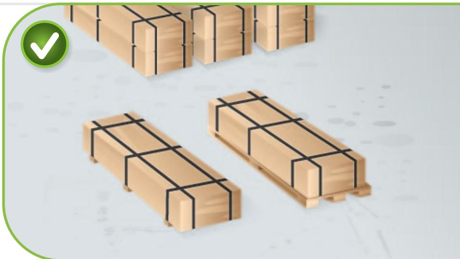
Store individual sheets on a stable basis over the ground. Use pallets, wooden strips or wooden bars-pads to avoid sagging of plywood sheets. ▶
