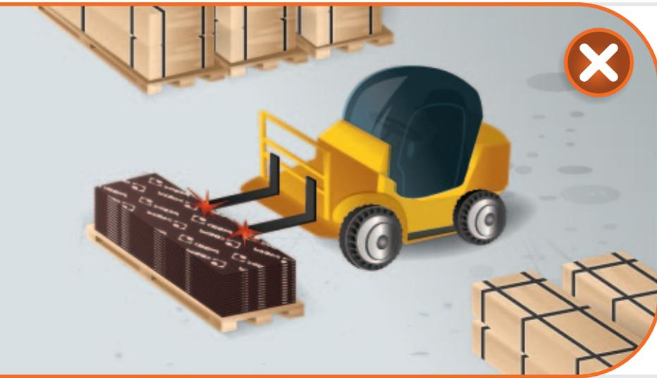
◀ Avoid damaging plywood sheets with loader pitchforks.
