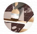
When cutting plywood, protect flat ends with paint. SVEZA recommends to use the acrylic paint TEKNOS Teknol JRL (Finland) or a sealant to prevent penetration of moisture (swelling).
