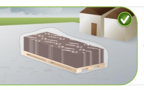
If plywood is temporarily stored outdoors, cover it with an impermeable material. Protect
