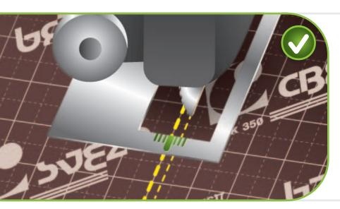
If the line of the potential cut does not match the markup line, use the blade on the saw panel. Put the blade in the cutting point.
