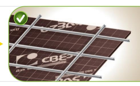
Put plastic chairs in required places. Determine the distance between chairs by grid cells.
