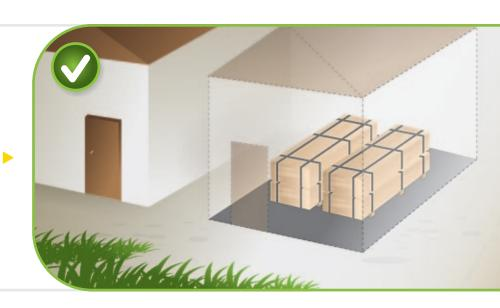
Plywood should be stored in a horizontal position, in the packs on pallets, wooden strips or wooden bars-pads (thickness – not less than 50 mm, length – not less than the width of a pack, without overhanging).
