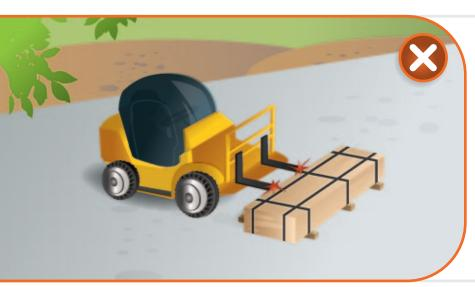
Do not push the packsof plywood with loader pitchforks.
