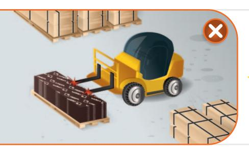
Avoid damaging plywood sheets with loader pitchforks.
