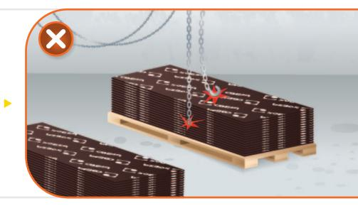
Remove sheets of plywood from the packs manually. Avoid damaging the flat ends, dropping plywood or dragging it over the ground.
