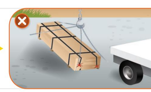
Metal straps, hooks or chains must not come into contact with sheets of plywood. They can touch only plywood side facings and covers of the packs.
